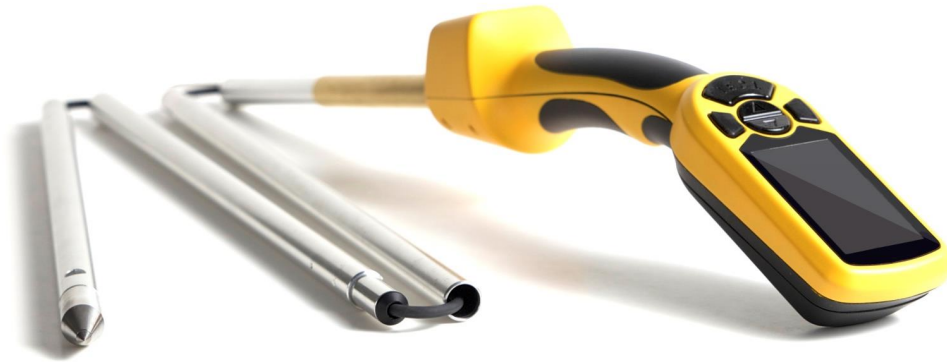
Figure 1a. Current version of AvatechSP, a collapsible digital snow profiler.
